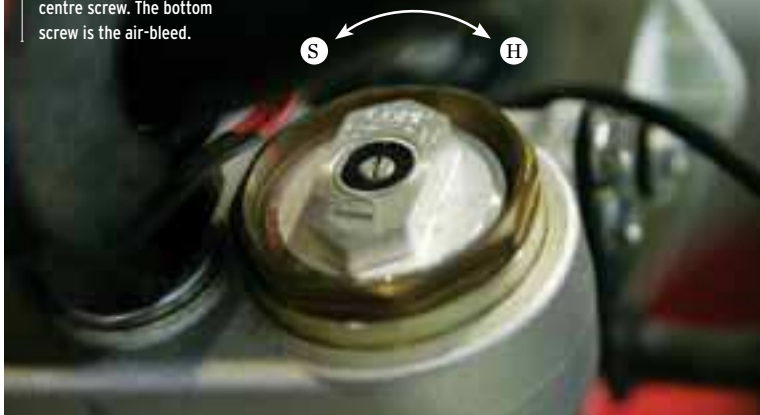
Shock adjustment showing high- (silver) and low-speed (red) compression.
